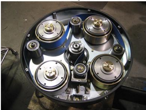
STEP 4 – Unscrew bolts to loosen Belt Tensioner.
